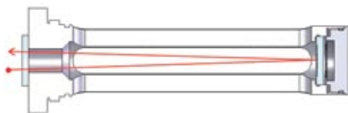
Figure 2: The passage of light into the SPECTRACAP® sensor probe used in the OMT300 series transmitters.
