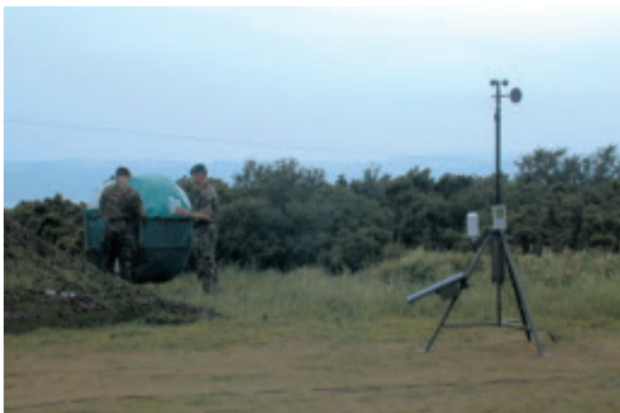
Performing an upper-air sounding using the mobile system, with the TACMET Weather Station directly connected to the upper air system.
