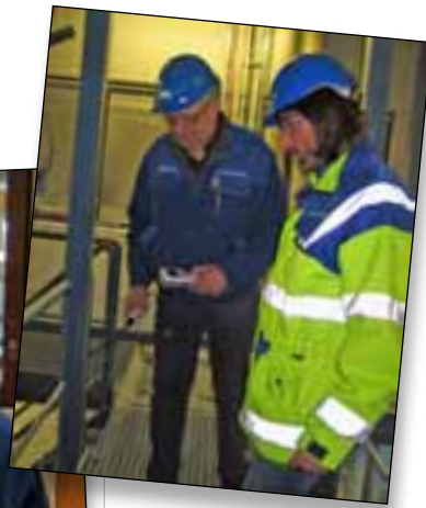
Reino Paloniemi and Jussi Nikkarinen use a Vaisala handheld humidity probe for spot-checking and configuring the measurements produced by the fixed humidity transmitters.
