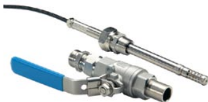
The MMT338 is ideal for installations in pressurized processes where the probe needs to be removed while the process is running. The probe depth is adjustable.
