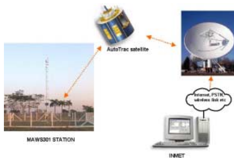
AutoTrac satellite offers two-way real-time access to the stations
