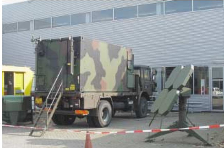
The radiotheodolite antenna tracks the radiosonde automatically throughout the sounding. An operator shelter on the vehicle is used for data processing and telecommunications equipment.
