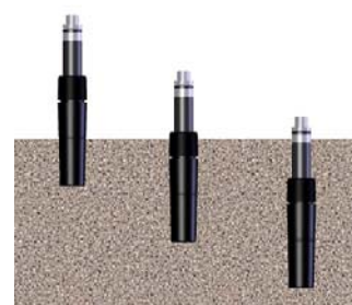
Figure 4. GMP222 probes in soil CO 2 profile
