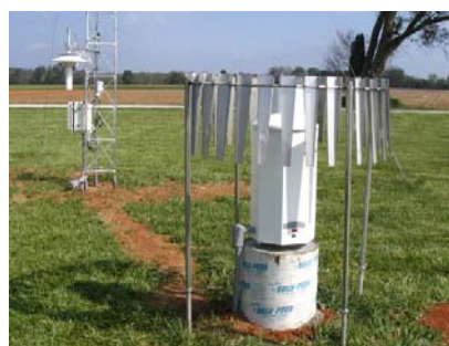
Figure 7. Vaisala Rain Gauge installed at the Bowling Green Mesonet station in the Kentucky Mesonet (photo courtesy Kentucky Mesonet).
