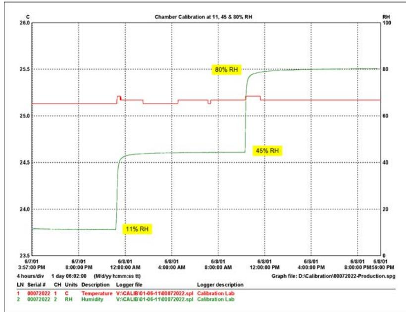
A typical 3-point data logger calibration cycle.
