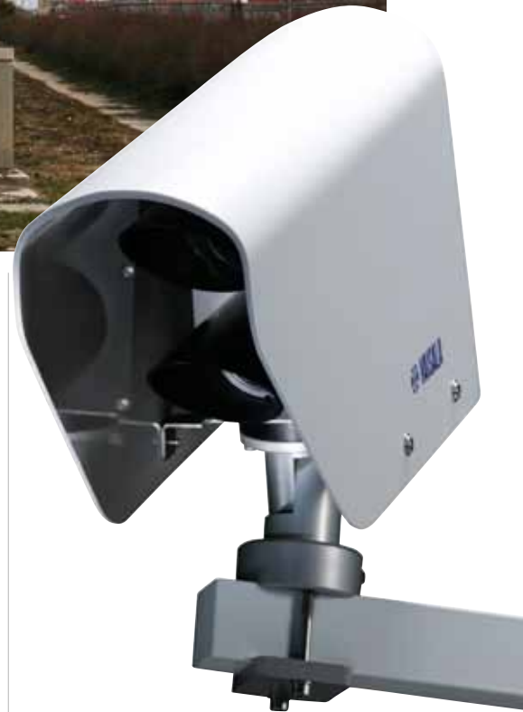
Remote road condition sensors monitor the Harris Overpass bridge surface, and automatically activate overhead mounted variable message signs to alert approaching vehicles of changing road conditions.
