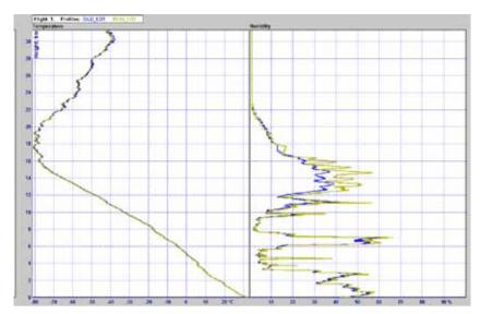
A day-time sounding profile from Malaysia, showing the effects of the improved algorithms on the humidity and temperature measurements.
