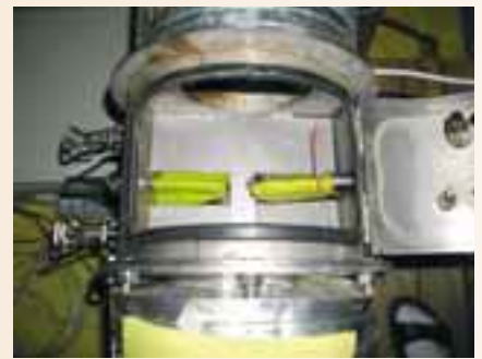
The wet bulb thermometer on the left is connected to the control system of the dryer and the one on the right is a psychrometer with a wet cloth.
