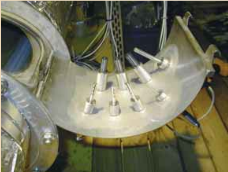
Placement of the sensors in the measurement drum's lock. Three Vaisala humidity probes, a Pentronic psychrometer and a WSAB psychrometer. The HMP247 Transmitters were installed in metal housing.
