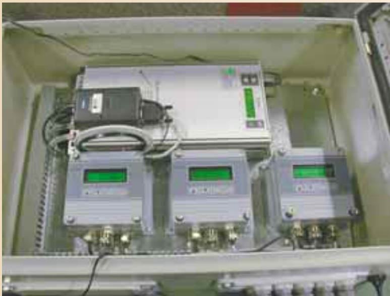
Placement of the sensors in the measurement drum's lock. Three Vaisala humidity probes, a Pentronic psychrometer and a WSAB psychrometer. The HMP247 Transmitters were installed in metal housing.
