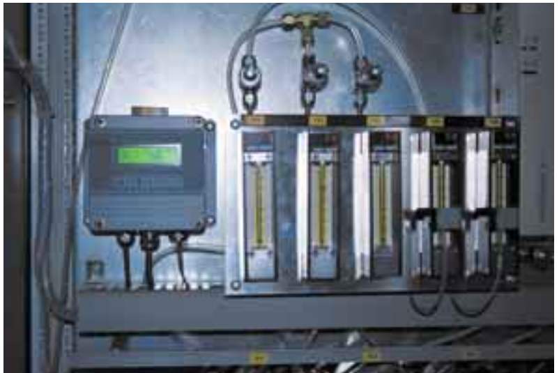
The Vaisala DRYCAP ® Dewpoint Transmitter DMP248 monitors dewpoint in an annealing furnace.
