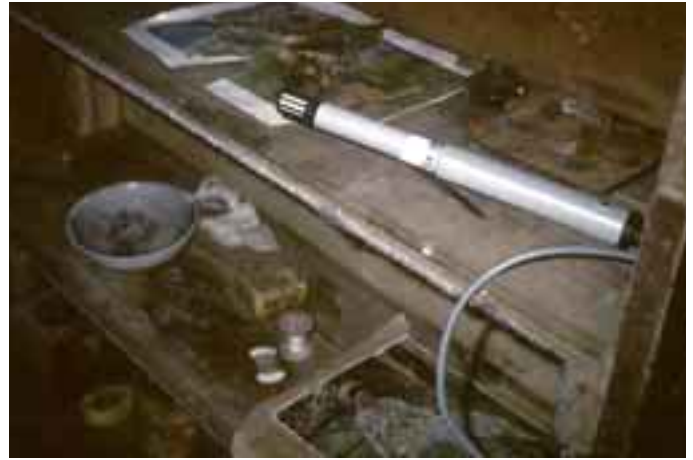
To further understand the deterioration processes affecting the building structure and artifacts, equipment for monitoring temperature and relative humidity, corrosion, salt deposition and erosion of timbers was installed in 1999.
