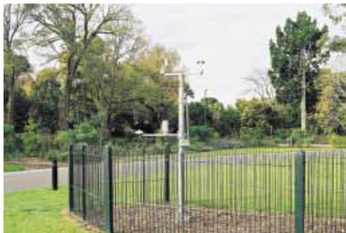
Vaisala's automatic weather station is equipped with sensors for wind speed and direction, temperature, relative humidity, solar radiation and rainfall.
