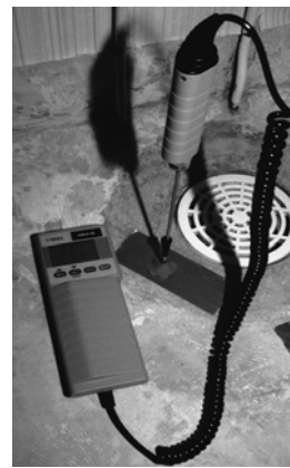
Figure 3.4.2 Taking measurements in concrete floors
