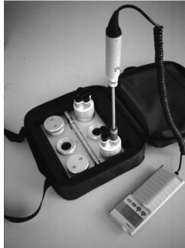
Figure 5.2.2 The HMP42 in a salt chamber of the HMK15 calibrator
