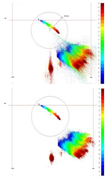
Fig. 2 Original and filtered LMA data on 2 Aug. 2013, 10:00 - 12:00 UTC, in the Kansas LMA, color-coded by time. The circle shows a 100-km radius around the center of the LMA. The two longitude lines are at -100 and -95 degrees, and the single latitude line is at 40 degrees.
