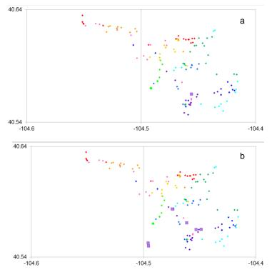
Fig. 6 Flash at 01:09:59 UT on 2013-09-23 in Colorado. Axes show latitude, longitude. Small dots are LMA sources, color-coded by time in 10 colors (purple to red). Larger squares are NLDN IC discharges. (a) without pulse train processing, (b) with pulse train processing
