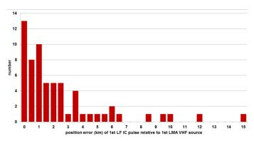
Fig. 4. Distribution of position errors between the first LMA sources and first pulses in pulse trains occurring at preliminary breakdown
