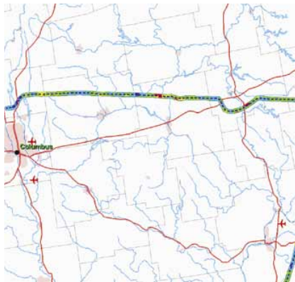
An example of a FALLS® 5.1 Exposure Analysis for a transmission circuit in eastern Ohio. Areas of higher lightning activity are revealed. This information can help an electric utility to prioritize protection or maintenance.
