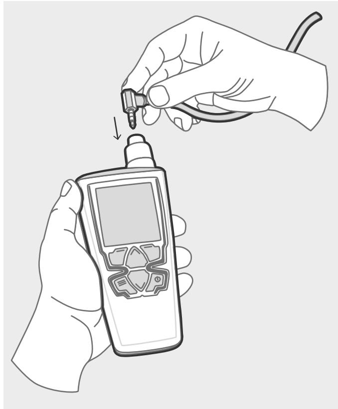
Connecting the HMP40S probe to the indicator quick connection adapter
