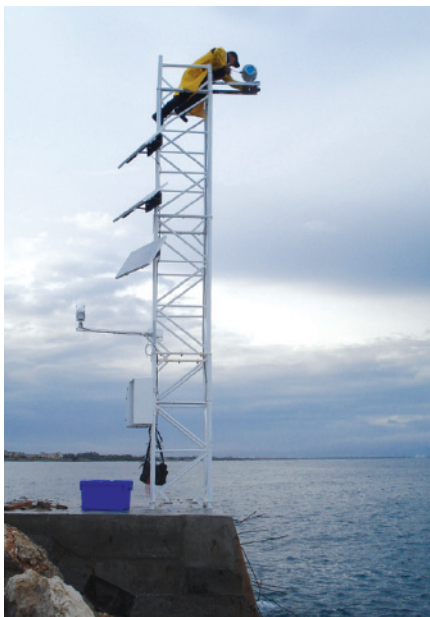
Vaisala Marine AWS with wave height measurement. Complies with IEC 60945 and Lloyd's maritime standards.
