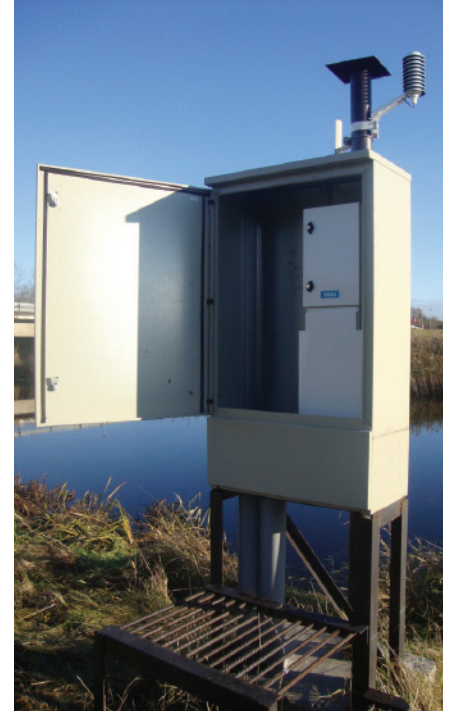
Vaisala MAWS Water Level Weather Station in Estonia. Vaisala Weather Radar is part of a complete hydrological system in Estonia.
