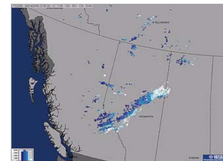
Vaisala LTS2005 Real-time Lightning Tracking Software maps CLDN data and provides estimated time of arrival to target locations and automatically monitors lightning activity in user-selected areas.
