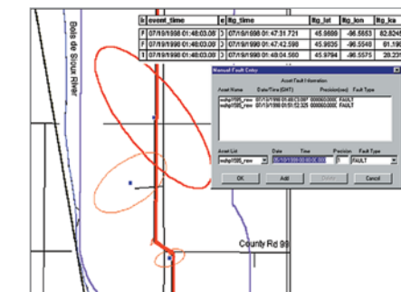
Vaisala's Fault Analysis and Lightning Location System (FALLS®) uses historic CLDN data to pinpoint lightning activity relative to outages and damage.
