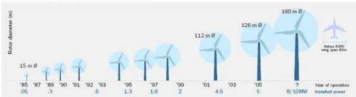
Figure 1: Size evolution of wind turbines over time. Source: European Wind Energy Association.
