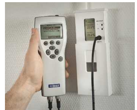
On-site calibration of a HMW90 humidity transmitter with a HM70 hand-held meter.
